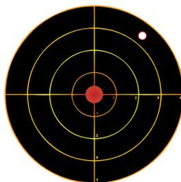
**Example:** Point-of-impact is 5" high and 3 1/2" right from aiming point. Use Correction Input: -19 D & -13 L
